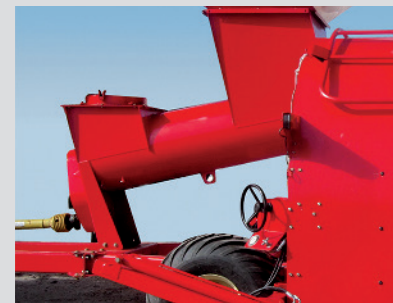
20" diameter auger for big loading capacity.
